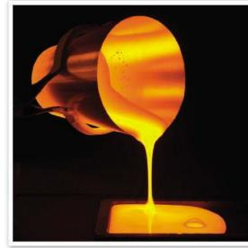
**Pouring it on.** Molten waste is poured from a platinum container as part of a process developed at Catholic University's Vitreous State Laboratory, built with a congressional earmark. (*Overleaf*) Lab director Ian Pegg holds a chunk of material after vitrification.
